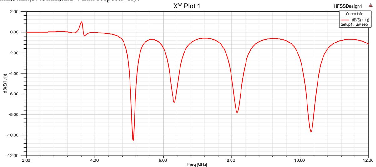
Fig. 2  $S_{11}$  vs frequency curve
